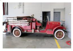
The original REO Speed Wagon, a regular truck, was purchased by the town of Hampton in 1924. In 1934, the Hampton Fire Department installed a Sanford Conversion kit, and the pumper remained in service in Hampton until 1955. The Pumper was then sold to Hampton Falls and remained in service until the mid-60s.
